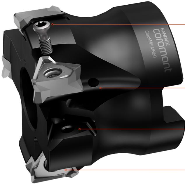
10IP TORX PLUS® screw to ensure 2 Nm (17.7 in-lb) tightening torque
