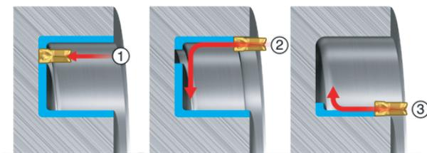
Make three cuts to separate material:
